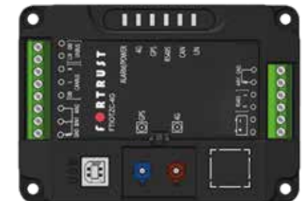
Control operator / Display panel
